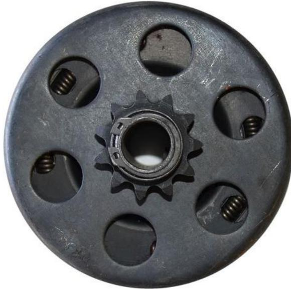
Centrifugal Clutch 5/8" bore 11 tooth #35 chain. does not come with set screws, if you need set screws you will need to order the Max-Torque clutch. **This clutch is designed to be held on by threading a bolt with a lock washer and fender washer onto the end of the crankshaft.**
